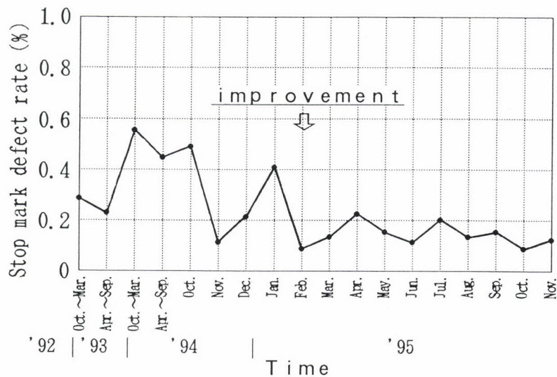
Fig.9. Variation in stop-mark defect rate.
