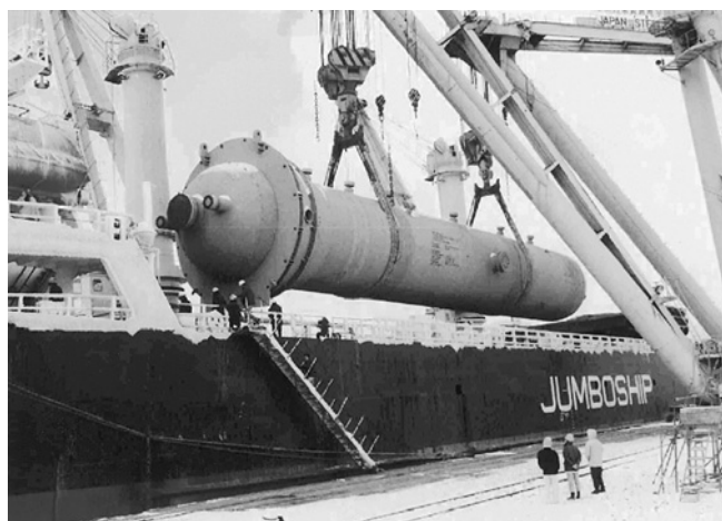
Fig.11 An 1450 ton weight hydroprocessing reactor
