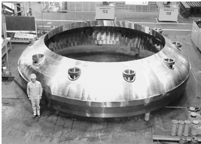
Fig.9 A component of ABWRPV made from a 600 ton ingot
