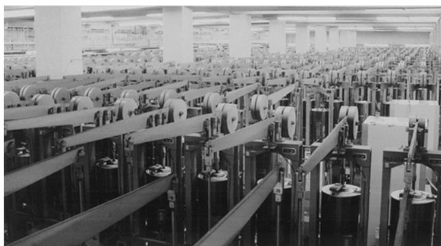
Figure 1 Creep testing machines in Meguro site
