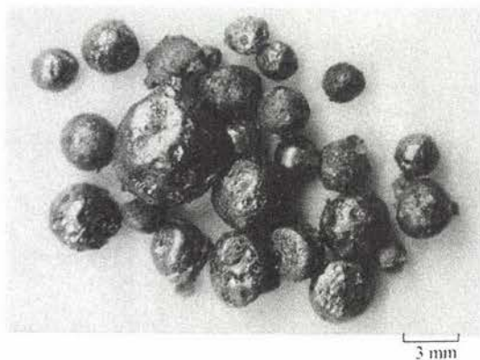
Fig.7 Particles of Fe-C-P alloy reduced from slag by microwave treatment 13) . (Treatment time = 7 min, Carbon equivalent = 1.5)
