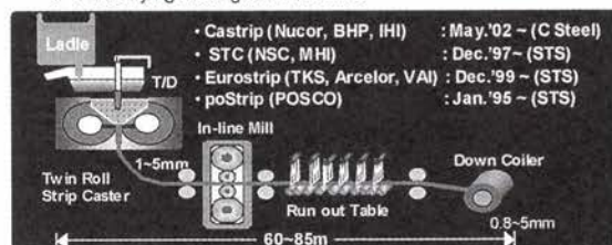
Fig.3 The Outline of Strip Casting Process.
