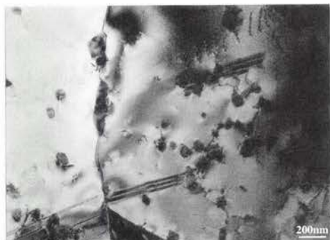
Fig.11 A TEM micrograph of 304H steel crept at 650°C with 98MPa and ruptured after 10558h
