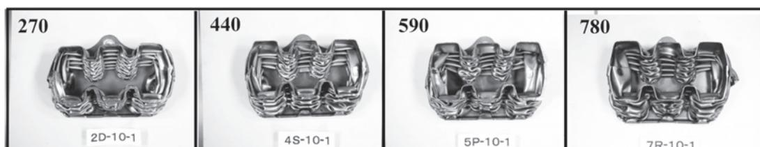
Fig.14 Deformed crash box with various steels after weight drop test
