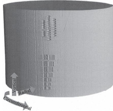
Fig.1 A resolution test object that has been prepared on a stainless-steel wire of  $497\mu\text{m}$  in diameter using the focused ion beam technique. The three arrows indicate three directions along which spatial resolution was measured.
