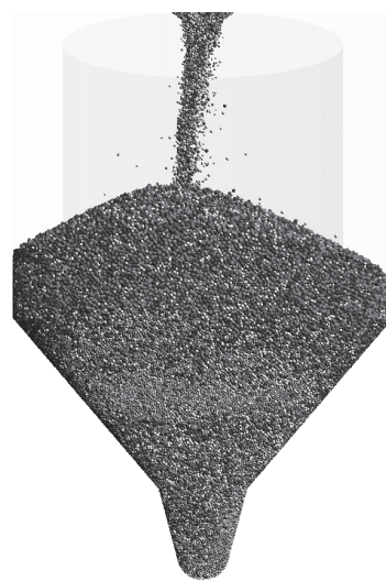
Fig.2 Snapshot of particle behavior charging into parallel hopper
