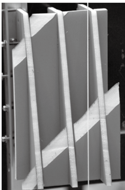
Fig.10 Cut model for ghost lines using foamed styrene. \theta = 15^\circ , \Phi = 90^\circ , \beta = 13^\circ .
