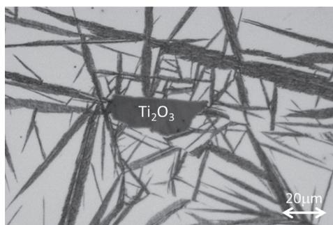
Fig.7 Bainite development after 4 hour holding at 300°C in  $Ti_2O_3$ -embedded superbainitic steel (Fe-0.8wt%C-1.6wt%Si-1.9wt%Mn-Cr,Mo)<sup>17)</sup>
