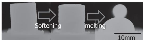
Fig.6 Shape of oxide tablet at softening and melting temperature.
