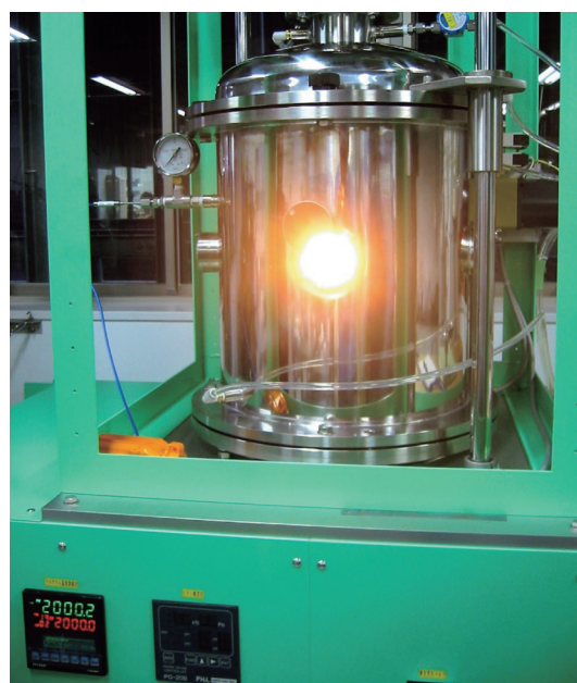
Fig.2 Appearance of the ultra-high temperature wetting furnace operating at 2000℃
