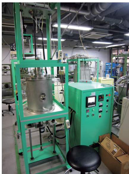
Fig.4 Appearance of the apparatus for simultaneous measurement of electrical capacitance and viscosity at elevated temperature.
