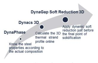
Fig.3 The Continuous Casting Model Suite
