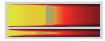
Fig.5 Calculated temperature of strand cross section(center view, enhanced colors indicating the mushy zone )
