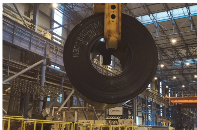
Fig.5 Arvedi ESP mill produced ultra-thin hot strip with a thickness of 0.6 millimeter.
