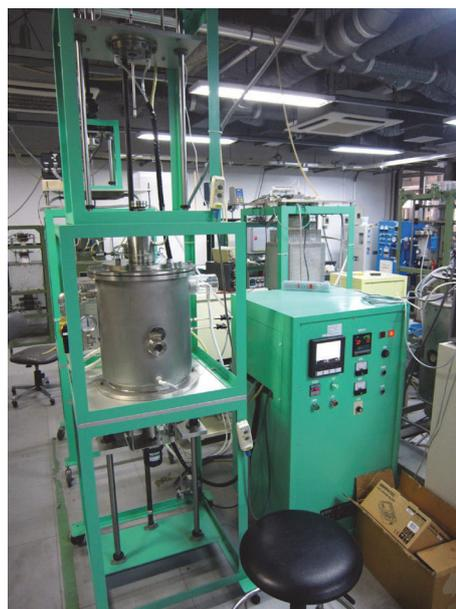
Fig.2 Appearance of the apparatus for simultaneous measurement of electrical capacitance and viscosity at elevated temperature.
