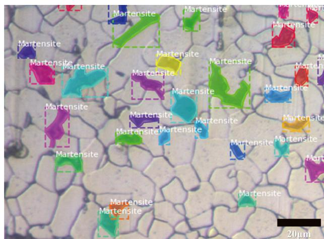
Fig.5 Segmentation by mask R-CNN<sup>®)</sup>.
