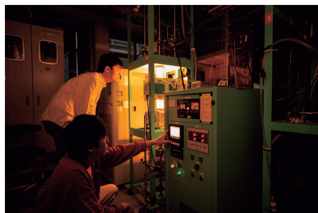
Fig.2 Experimental scenery with softening and melting test of iron ore under high temperature conditions. (Online version in color.)
