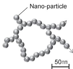
Reducing thermal conduction through Nano-particle network by minimizing contacting area.
